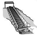
the government. Fish can safely swim past the cylinder on their way down the river, while 'fish ladders' can be provided to help fish cross weirs when travelling upstream.
